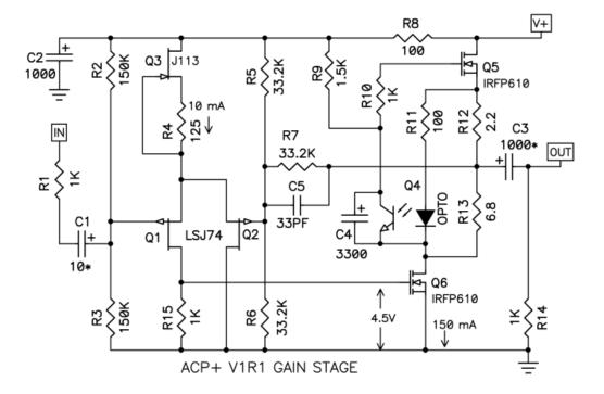
Figure 1. Original ACP+ Line Stage circuit.
